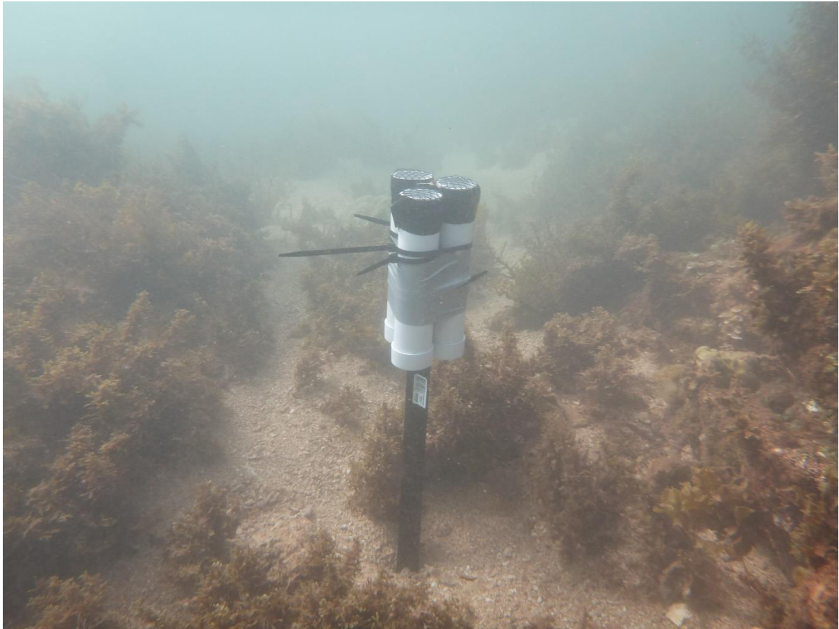
Figure 2: Sediment tube traps in situ at site Eva north offshore. Two clusters of three traps were deployed at each site.
